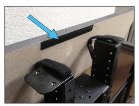
Step 2: LID PROTECTION -- Line the underside of the cabinet lid with the 6 ¾" soft Velcro strip directly behind the Screen Support Bracket. You may also place Velcro strips along the bottom section of the Hinged Top Guide bracket to provide additional protection. Placing Velcro strips along both the lid and Hinged Top Guide Bracket ensure the lid is protected while it travels against the back of the Screen Support Bracket.
