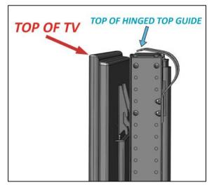
**Step 3:** Install the TV  $\frac{1}{2}$ " below the top of the Hinged Top Guides, so that the cabinet lid does not touch the TV during operation. You may bend the Hinged-Top Guides up or down slightly to achieve this tolerance.
