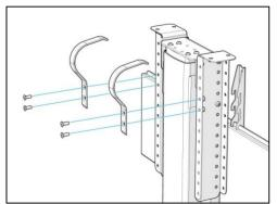
**Step 1:** Attach the Hinged-Top Guides, as shown in photo at left, to the slotted holes on the back of the Top Support Brackets. Secure them by using the four (4) 6mm x 12mm Flat Head machine screws and 6mm Nyloc nuts.
